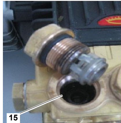
O-Ring in valve seat
