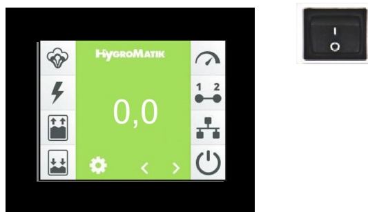
Touchscreen and main switch
