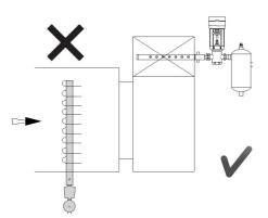
The minimum distance between the steam lance and the duct humidifier controller should be at least 5x the humidification distance.
