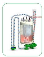
Depending on requirements, HyFlush and HyCool can also be installed individually. In addition, all units of the FlexLine series can be equipped with a **stub line flush**, which prevents contamination of the supply line by standing water during longer idle periods in accordance with VDI 6022.
