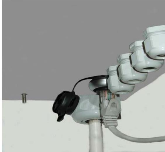
Connection of the RJ45 cable to the plug on the bottom side of the steam generator housing
