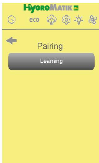
If subsequently a new remote control is to be connected to the steam generator, then this remote control has to be registered at first.
