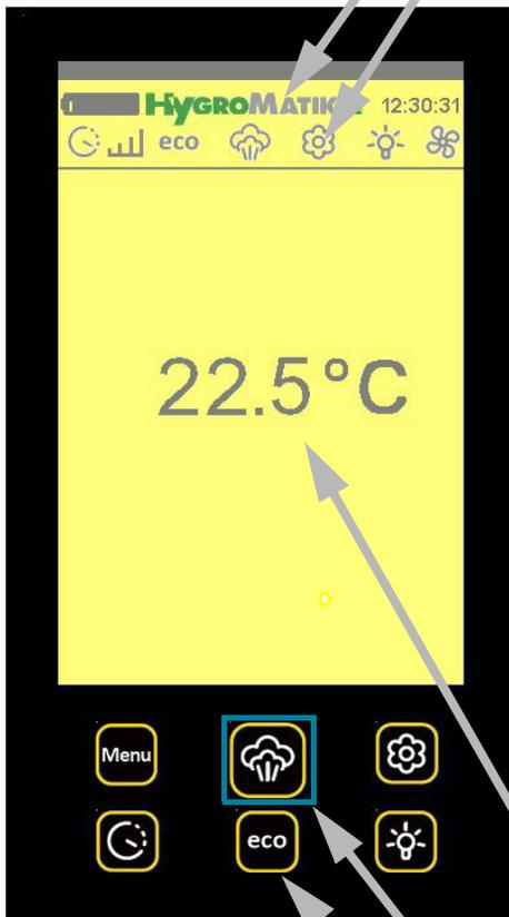
The current actual temperature in the steam bath. Improper temperature values are indicated by arrows showing up or down. This area also is the touch screen interface. Operating menus and submenus for the setting of parameters are displayed here.
