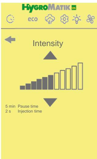
Factory setting is 6 bars corresponding to an injection time of 2 seconds and a pause time of 5 minutes. Setting less bars will increase the pause time whereas the setting of more bars will increase the injection time.
