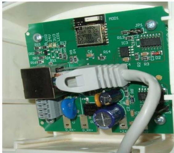
Connection of the RJ45 cable to the charging cradle electronics
