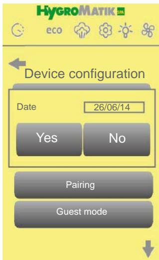
This menu allows for setting time and date of the steam generator control.
