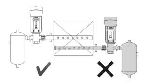
If the humidifier blows into a compact multi-zone unit then it should be installed directly in the air flow and as close as possible to the fan.
