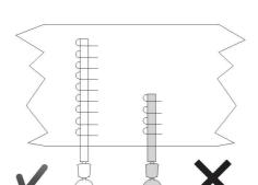
The bifurcated pipe should never be installed less than one meter in front of the fan suction side. In this case the correct installation is behind the fan.
