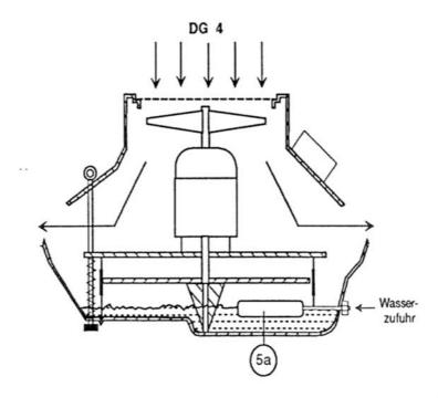
The waterlevel in the base tube is controlled by the lower flow switch of the two-step flow switch.
