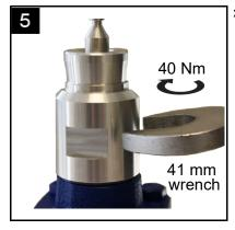
Screw on adapter on valve bonnet and fasten with a 41 mm width across flats wrench (set torque to 40 Nm).
